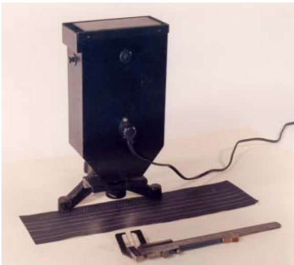
Figure 12: The original aids from Franz Wethlo for easier interpretation of the recorded waveforms. This equipment consisting of a measuring projector and a vernier gauge is now in the historic collection of the Dresden University (from [19]).
