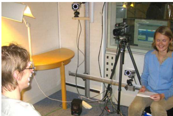
Figure 1: Data collection setup with video and IR-cameras, microphone and a screen for prompts.
