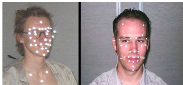
Figure 2: Test subjects with the IR-reflecting markers
