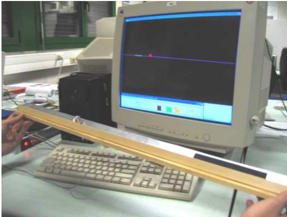
Figure 1: The Ballancer with a 19" graphical display. The simultaneous use of the real glass marble on the track and the virtual ball on the computer screen only serves for demonstration purposes in the photo. All test settings contain only one of the two elements, "real" or virtual ball.
