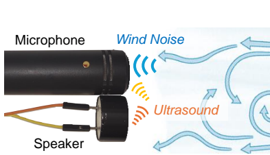
Figure 1: DeWinder uses ultrasound to sense and reduce wind noise.
