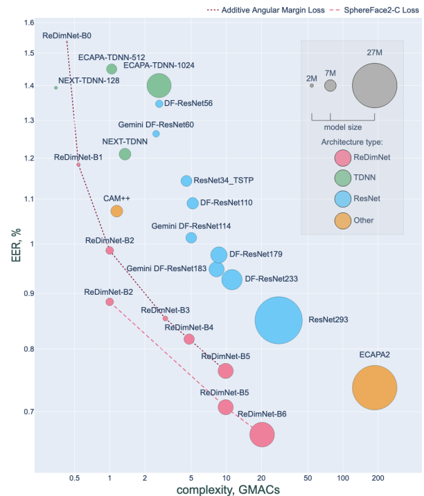
Fig. 1 Computational Cost vs. Average Equal Error Rate. EER is averaged over three Voxceleb1 protocols: Vox1-O, Vox1-E, Vox1-H. The model size is shown by the area of a circle, model family is indicated by a color. Complexity is assessed using thop library with an input signal of 2 seconds. A short dashed line represents scaling the ReDimNet architecture using the Additive Angular Margin loss function [19], dashed line - using the SphereFace2 loss [20].
