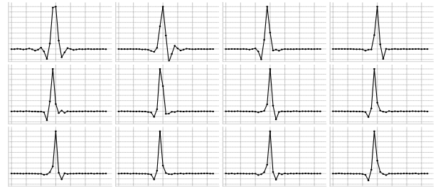
Figure 3: Visualizing the first 12 rows in Figure 2 (left), i.e. 1D temporal convolutional filters of width 33 in the first temporal convolution in QuartzNet after training. The Y-axis range is [-0.3, 1.1] for all plots. All filters are very similar.
