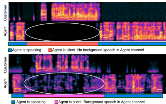
Figure 1: Spectrograms (in oval) showing presence or absence of background speech in the Agent channel
