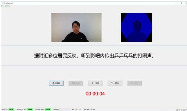
Figure 2: The main acquisition interface of the C#-based data acquisition system, which simultaneously acquires RGB color images, depth images and audio signals.
