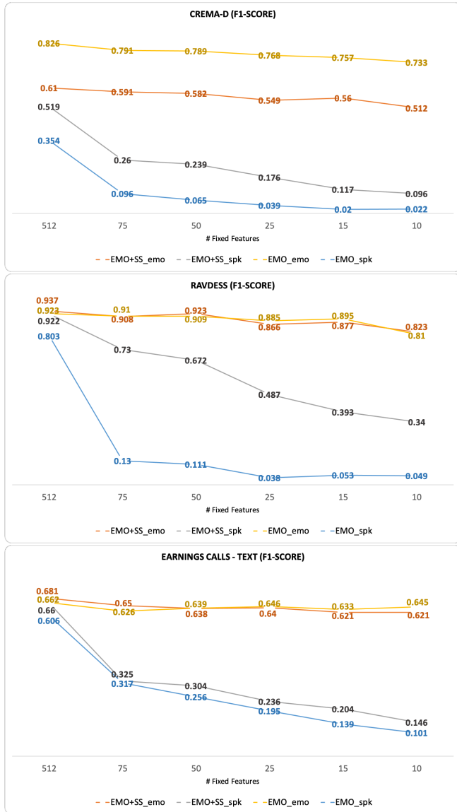
Figure 3: Suppression of speaker identification after embeddings shuffling. We show the number of fixed (unshuffled embedding dimensions) on the x-axis, ranging from 512 (no shuffling) to 10 (502 features shuffled). (i) EMO + SS emo (dark orange) is F1-score for emotion detection based on adversarial training embeddings; (ii) EMO emo (dark yellow) is for emotion detection w/o adversarial training; (iii) EMO + SS spk (dark grey) is F1-score for speaker identification with adversarial training; (iv) EMO spk (blue) is for speaker identification w/o adversarial training.
