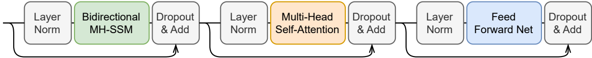
Figure 4: Stateformer: Bidirectional state space augmented transformer block. It simply has an additional block prior to the attention unit with a bidirectional MH-SSM. The pure MH-SSM architecture is similar but without the self-attention block.
