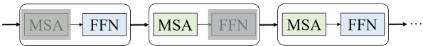
Figure 3: A conceptual overview of our method. A sub-module may be completely removed (e.g. shadowed blocks) from the downstream model by using the BAS strategy.
