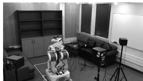
Figure 2: The experimental setup used to record RIRs.
