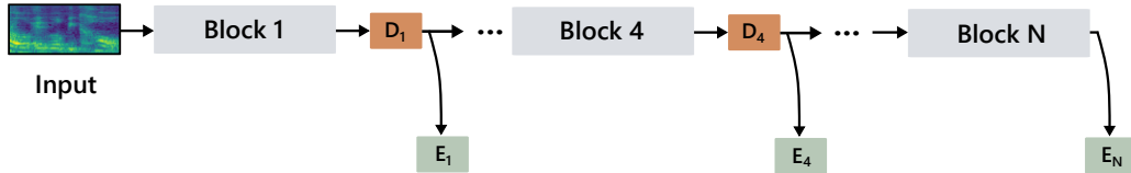
Figure 1: Overview of our early-exit binary neural networks. Grey blocks denote a set of binarized convolutional and other layers, orange and green squares denote decision exits and classification output layers, respectively. Our early-exit model enables adaptive inference for each input sample based on an entropy-based decision threshold to early-exit the input, thus saving computation.
