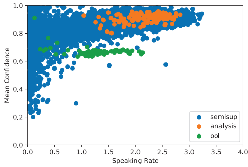
Figure 1: Plotting speaking rate against mean lattice confidence for each utterance in: our raw Youtube data (‘semisup’); our analysis data-set; and out-of-language data (‘ool’).
