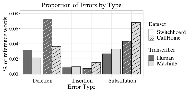
Figure 1: Proportion of errors of each type as a total of the reference tokens.
