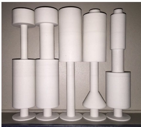
Figure 1: Set of VTM-T20 models (/i/, /e/, /a/, /o/, and /u/ from the left). They are designed based on VTM-N20 models originally from Chiba and Kajiyama's measurements and simplifications [4]. Further simplifications were applied to achieve the VTM-T20 designs for pedagogical purposes.
