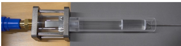
Figure 3: VTM-S24 model. Instead of the 40-mm diameter and 170-mm or 190-mm length used for VTM-S20 model, the diameter is 24 mm, and the length of the outer tube is 145 mm.
