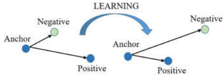
Figure 3. The Triplet Loss minimizes the distance between an anchor and a positive, and maximizes the distance between the anchor and a negative [12].
