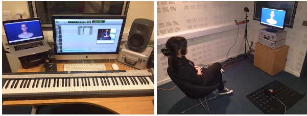
Figure 1: The researcher's WoZ setup on the left, the participant setup on the right
