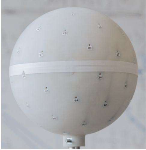
Figure 1: 64-channel spherical microphone array, allowing a 7-th order spherical harmonic approximation to the recorded sound field.
