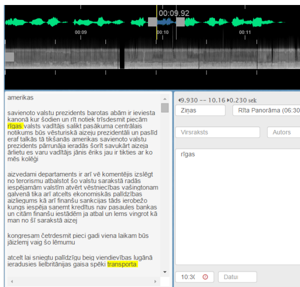
Figure 2: The user interface of the system, containing audio waveform, spectrogram, ASR output and highlighted keywords.
