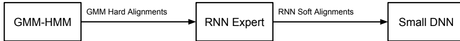
Figure 1: We use the hard GMM alignments to first train a RNN, after which we use the soft alignments from the RNN to train our small DNN.
