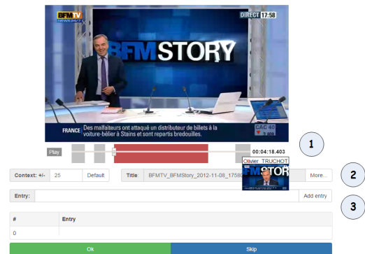
Figure 2: Overview of the web front-end UI. 1) Video player displaying the track to annotate and the synchronized context bar . The red glyph shows the track to annotate, and additional annotations appear in light gray. 2) The context bar configuration and the metadata field. The latter displays the video title, and reveals additional details when activated. 3) The textfield to type the annotation. Multiple annotations are supported, and summarized in a table.
