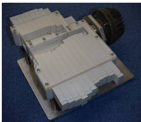
Figure 1: Umeda and Teranishi's model. A set of plastic plates are inserted from the side.
