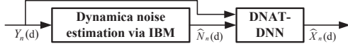
Figure 2: A block diagram of the proposed two stages of DNAT based on the dynamic noise estimation via IBM.
