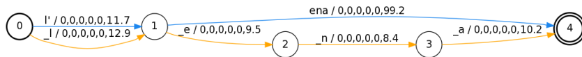
Figure 2: Example of a lexical-phonetic automaton : accepting the lexical path “l ena”, the phonetic path “l _E _n _a”, and the lexical-phonetic paths “l _E _n _a” and “l ena”; and weighted by a vector of 6 different features.
