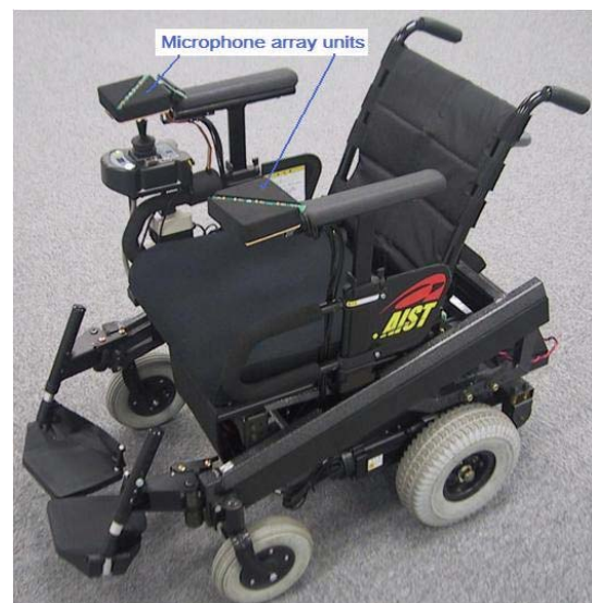
Figure 1: A wheelchair with the microphone array.
