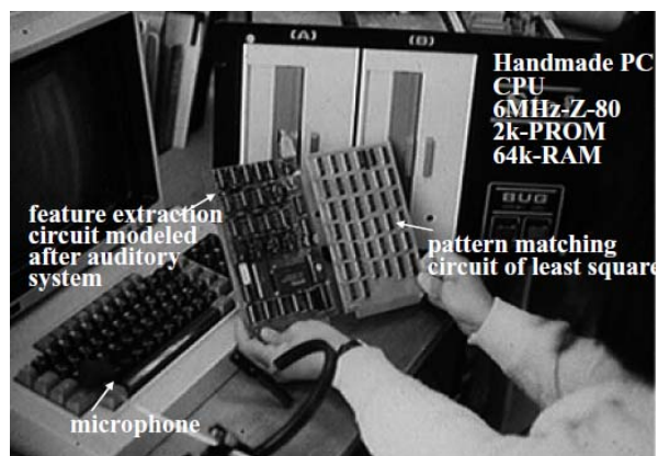
Figure 8: Monosyllabic voice typewriter using a Z80 microprocessor and 32kbyte memories.
