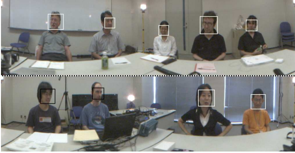
Figure 3: Typical output from the program showing two 180 degrees sections on top of each other. Detected faces are shown with a white square, tracked faces with a black square.
