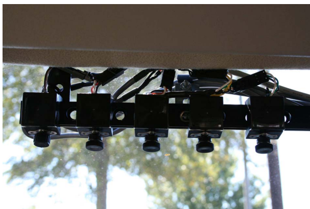
Figure 1: Custom-designed adjustable-spaced microphone array.
