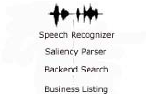
Figure 1: An overview of the directory-assistance system showing the role of the saliency parser.
