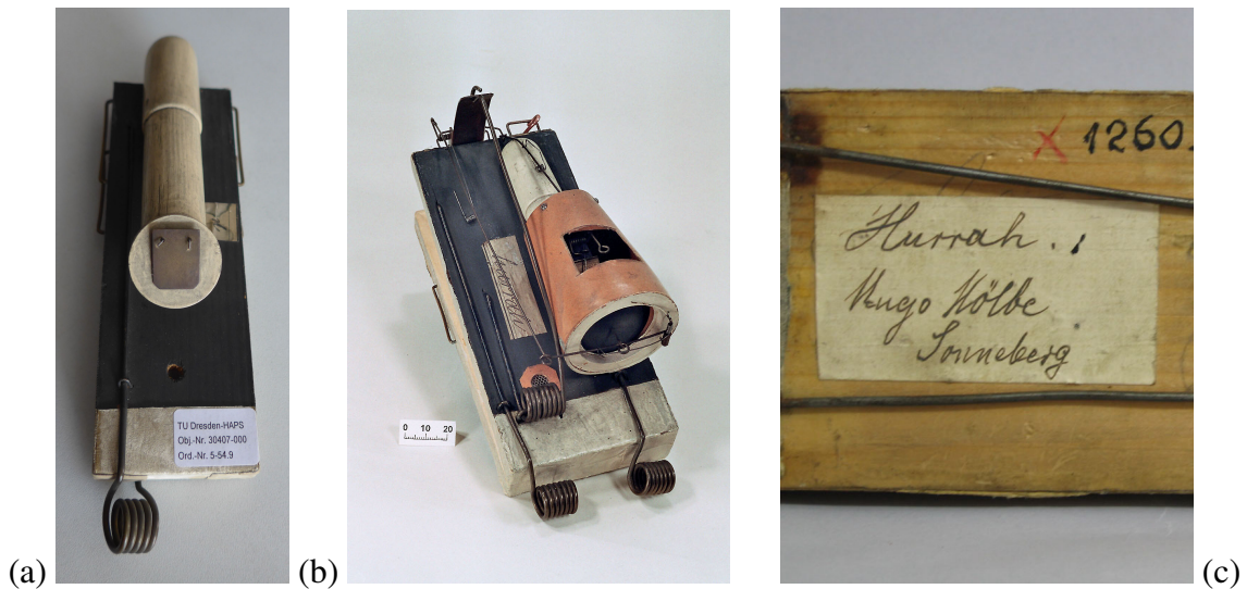
Figure 5 - The Hurra voice from Hugo Hölbe. (a) Voice for producing the consonant r separately. HAPS Dresden. (b) Voice for producing the word Hurra . HAPS Dresden, photograph by Rolf Dietzel. (c) Signature of Hölbe at the underside of the Hurra voice in the collection of the Deutsches Spielzeugmuseum Sonneberg. Photograph from a visit in February 2007.
