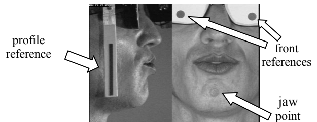
Figure 2: Video signal recorded: measurement method.
