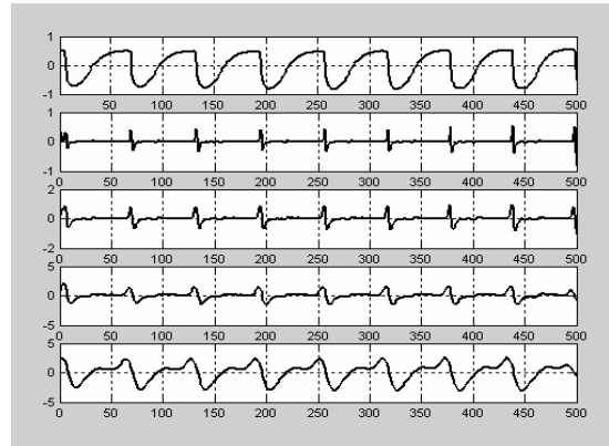
Figure 2: Wavelet transform of EGG signal (wavelet with 2 vanishing moments) for different values of scale varying from 2^3 to 2^0 . at the top of the figure, we find the EGG signal followed by its wavelet transforms.
